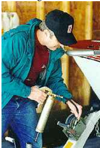
Inspect, clean and grease cables to keep winches moving smoothly. Bob Queen, © 1998
